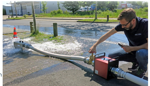
1) Preparation for separate turbidity measurement HTL TE / TU
