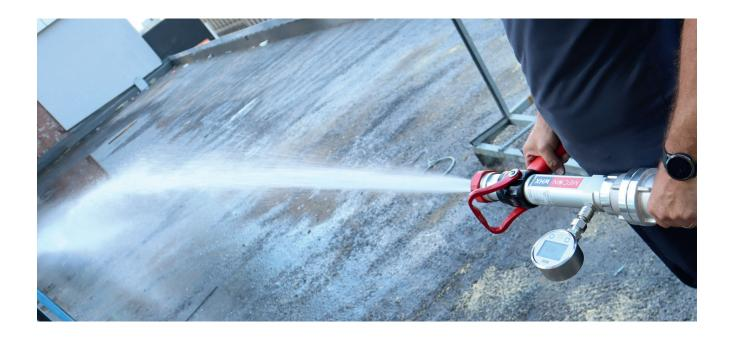
The fire hose reel tester WHX was specifically developed for testing wall hydrants hose reels of types F and S according to DIN 14462:2023-07. The testing device enables precise measurement of the defined ranges from 24 I/min at 2 bar ... 600 I/min at 4.5 bar (6.3 USgpm at 29 psi ... 159 USgpm at 65.3 psi), taking into account simultaneous usage.
